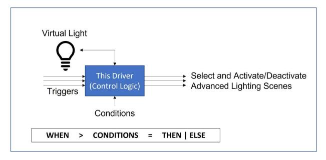
The driver implements a 'WHEN > CONDITIONS = THEN | ELSE' model. In other words, the driver is usually triggered by a user or system action, such as the user pressing a keypad button, a contact being activated (a door being opened, for example), the driver's own Virtual light being turned ON or a programming command being issued. This is the WHEN part.
