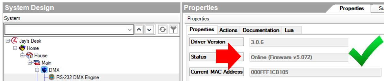
**Do NOT use Core5 DB9 ports or HC-250 Serial Ports! Only 3.5mm serial port will work on Core5. Any other controller should work perfectly. Don't ask me why...**
