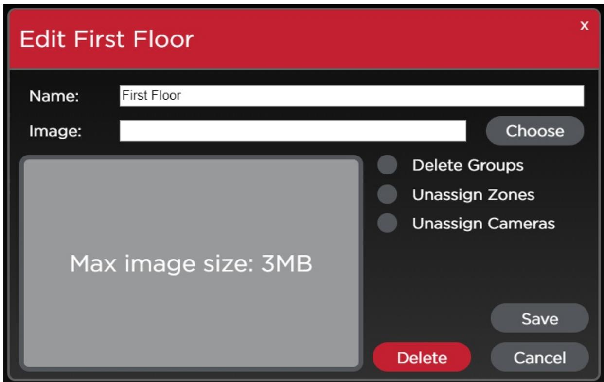
You can define the name of this area, and choose an image to be displayed in the background (usually a floor plan). When choosing an image, keep in mind that the image will be stretched to occupy the entire space of the touch panel, which has dimensions 962x551 (roughly 16:9). Using an image of roughly that aspect ratio will minimise any potential distortion.
