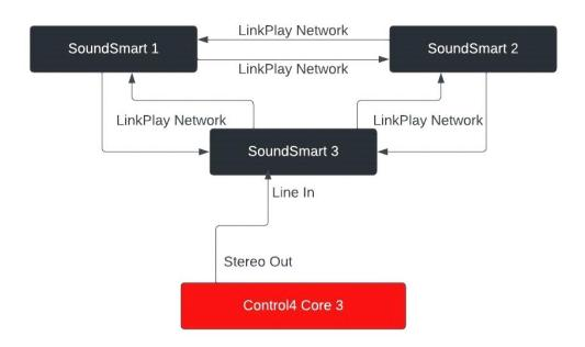
Note that a controller connected to one of them (TV or any audio source) can be distributed to the others via the network.
