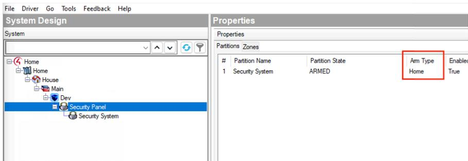
If this is not the case, you can use the **Partition State** mode where you can manually set the partitions to monitor (set below) that will uniquely distinguish between the **Home**, **Away**, and **Night** armed states. For example, if you have an "Interior" and "Perimeter" partition, you would select both partitions for the **Away** state and only the "Perimeter" partition for the **Home** state:
