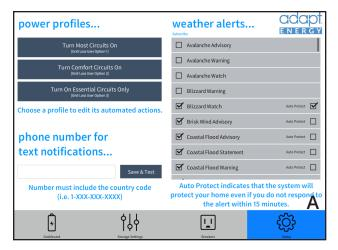
On the Settings dashboard, enter the phone number(s) on which you want to receive text notifications. Multiple numbers can be entered using comma separators. Click Save and Test to send a test message to all numbers listed.
