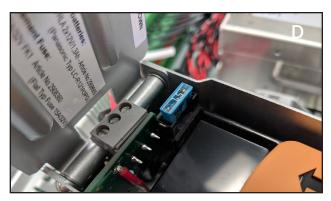
Close the case and re-mount the UPS battery on the DIN-RAIL.
