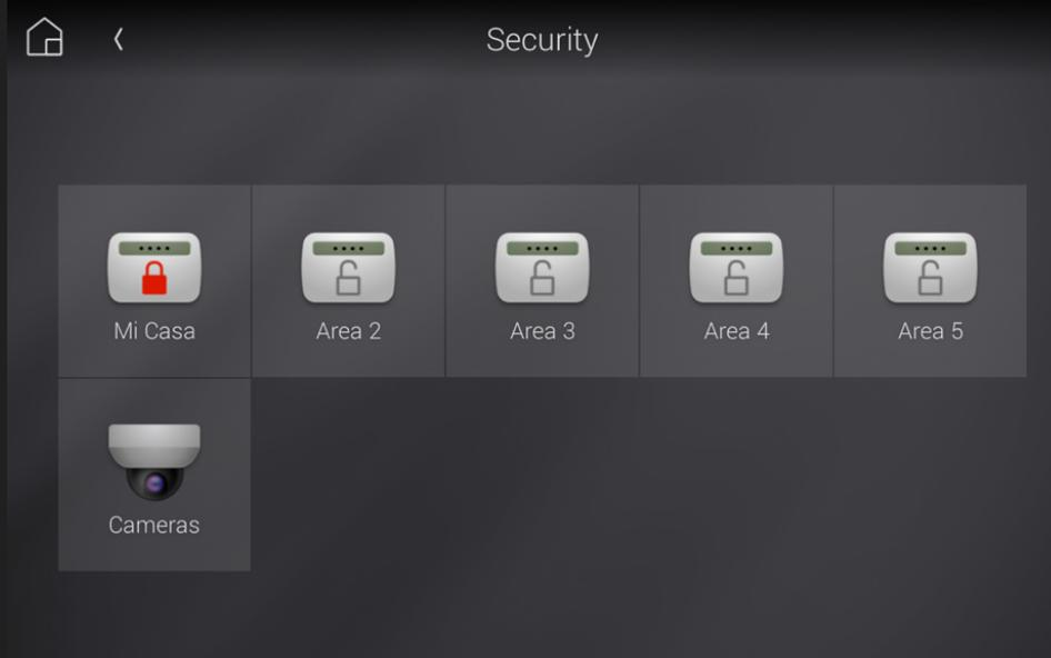
Each partition keypad had the ability to arm, disarm, execute emergency actions and trigger specific functions. Click on the center circle to choose different arm settings or disarm the alarm. If Arming and *Quick Arm Enabled* is activated, the driver will immediately try to arm the system when asked to arm. If not, the user will need to enter their 4 or 6 digit access code.
